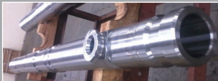
SS 403 MODIFIED IN END FITTING IN FINISHED MACHINED CONDITION
