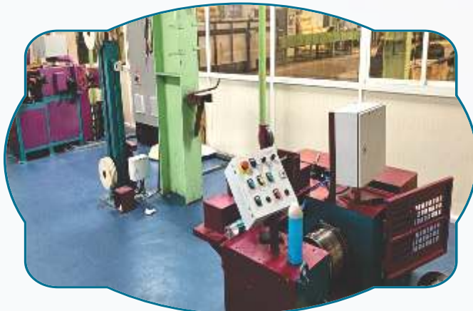
Layer Winding Machine: This machine is used for layer winding of fine GMAW wires.
