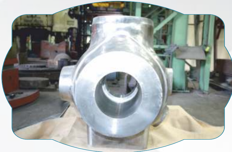
High pressure valve casing for AUSC made of Nickel based super alloy (SN 617CC) through open die forging
