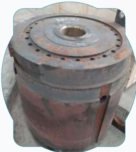
195 Dia container made of Iron based super alloy SF 286 & adaptor
