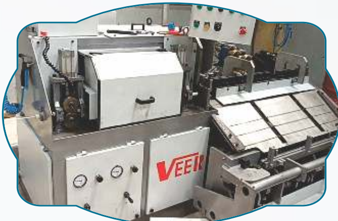
Straightening, cutting and embossing machine for manufacturing of TIG/GTAW wires.
