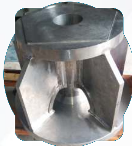
Adaptor (made of Titanium Grade 9) is a critical component for assembly and requires load bearing capacity for different shock and load conditions
