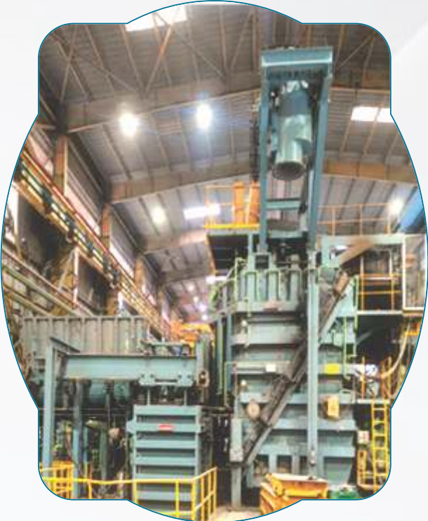
Vaccum Induction Melting Furnace (VIM)
