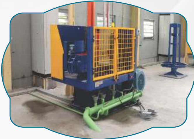
760 MM Single head Bull Block machines for cold wire drawing operation
