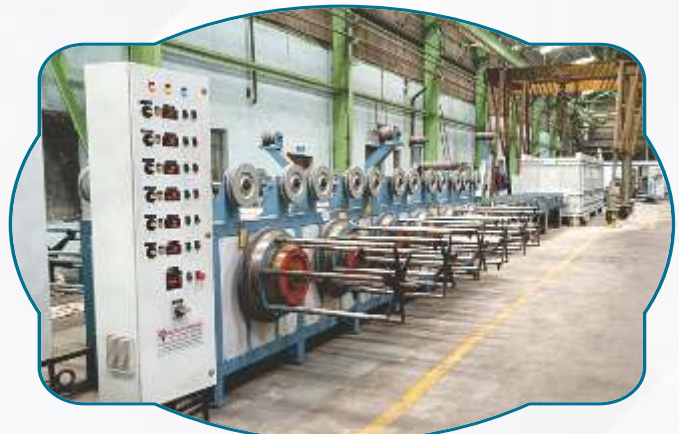
Bright annealing furnace/continuous annealing furnace. maximum annealing temperature: 1150°C Annealing will be done in protective atmosphere with pure Hydrogen gas.
