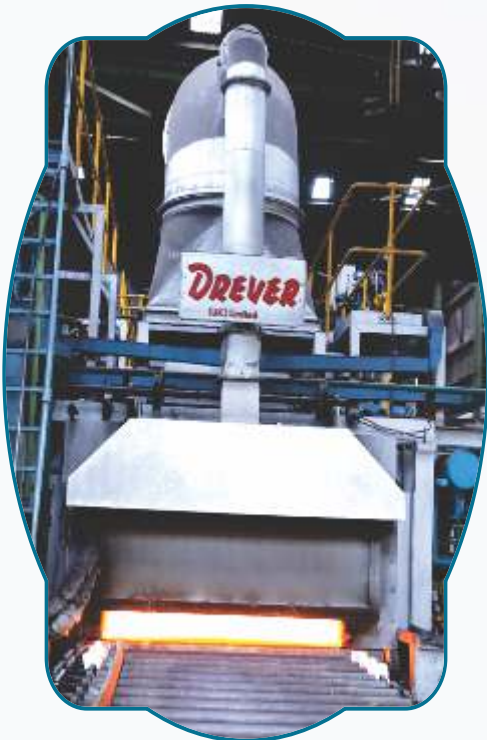
Roller Hearth Furnace
